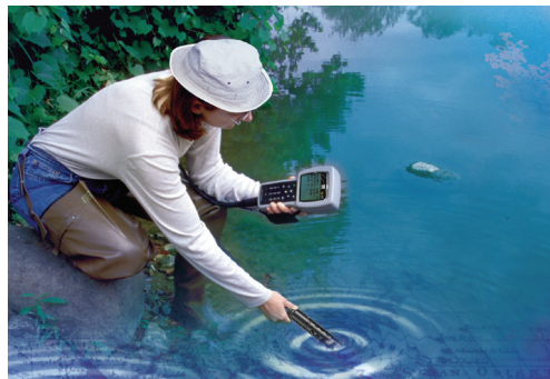
The YSI 556 MPS handheld display instrument measures several water quality parameters, logs data, connects to a PC, is waterproof, and has a 3-year warranty.
